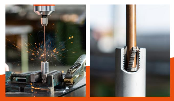
The hollow copper electrode is clamped in the oscillating head. It is smaller in diameter than the broken-off tool. During the erosion process, the core of the broken-off tool is vaporised by spark discharge. Vaporisation releases the cutting edges and allows them to be easily removed. The electrode does not come into contact with the workpiece, meaning that the thread remains undamaged. The company's standard choice of drilling emulsion is used as the coolant.
